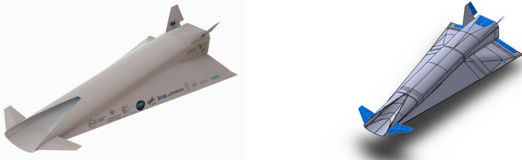
Fig. 1. The STRATOFly MR3 aircraft concept rendering (left) [8] with details on control surfaces (right)
