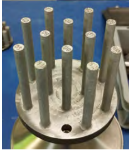
Fig. 4.48 PBF-LB/M cylindrical blanks used for the machining of tensile specimens. The blanks shown in the figure were produced in the vertical orientation, with their longitudinal axis parallel to the build-direction axis ( Z ) of the PBF-LB/M system. After heat treatment, when required, the final cylindrical tensile specimens were obtained by turning.
