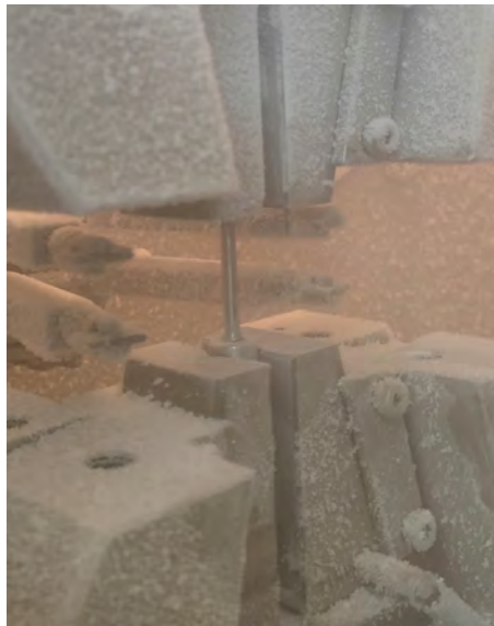
Fig. 4.51 Low-temperature tensile test setup used for testing the PBF-LB/M UNS S32760 specimens at -46\text{ }^{\circ}\text{C} . The specimen was mounted in the grips of the tensile testing machine inside the climatic chamber and acclimatized for an additional 15 min before testing, in order to ensure thermal stabilization under the selected test conditions. The specimen temperature was monitored throughout the entire test by means of a thermocouple.
