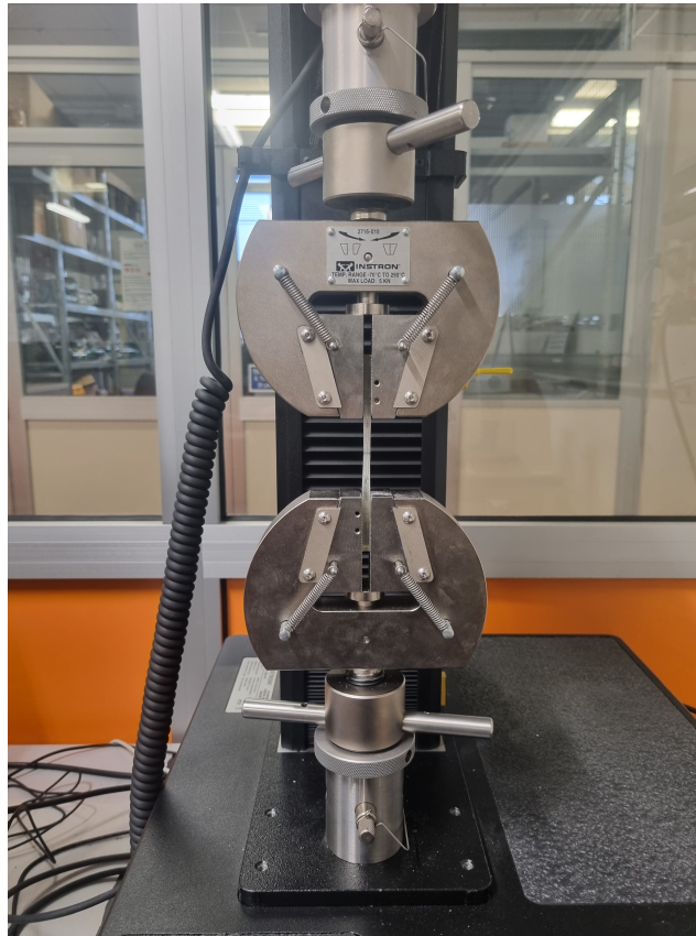
Fig. 3.13 Transverse Fiber Bundle Test [0°] on CF/epoxy specimen.
