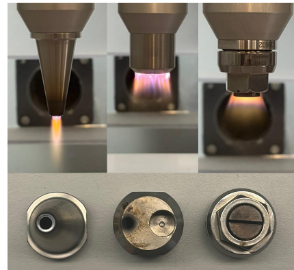
(b) Front and up view of equivalent Plasmatreat configurations, from left to right: straight, rotating, static blade-like (8 mm width, selected for UD).
