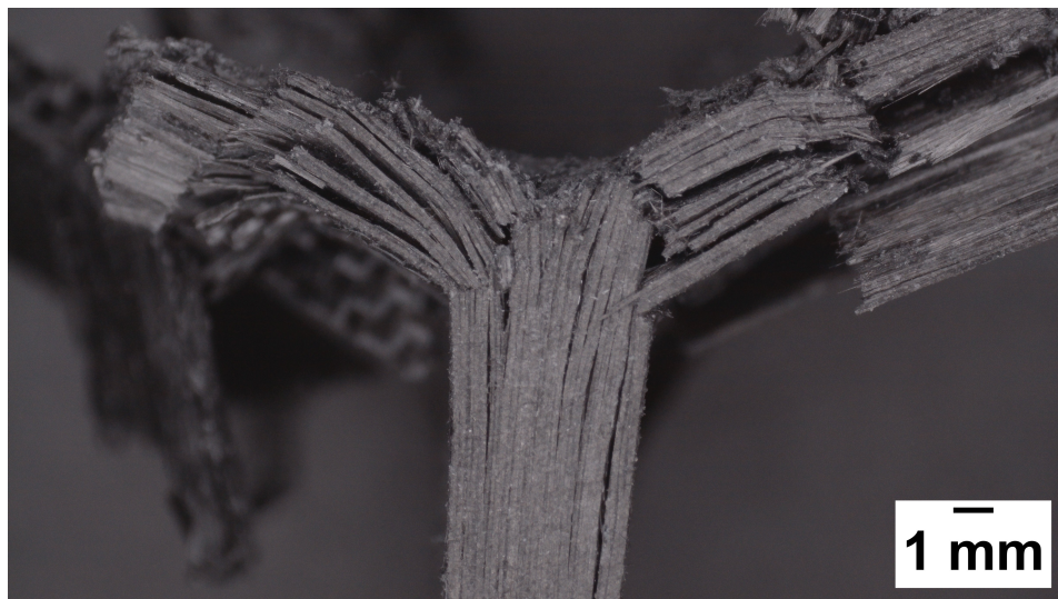
Fig. 6.15 Detail of the splaying mechanism and frond formation in the crush zone.
