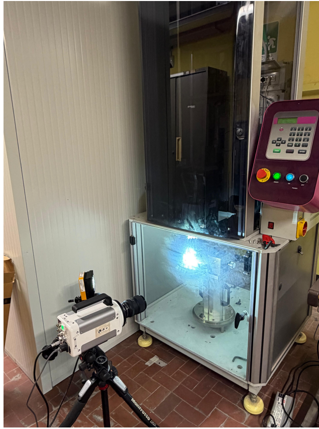
Fig. 3.16 Instron Fractovis drop dart machine test and High resolution and acquisition camera.
