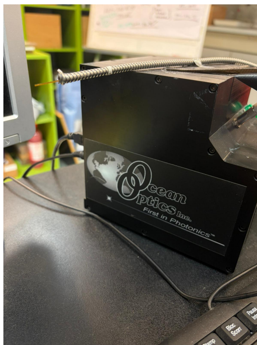
Fig. 3.6 Ocean Optics LIBS2500+ spectrometer equipped with fiber optic probe.
