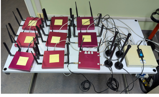
Fig. 1: Laboratory setup with nine OBUs. Each device hosts three TRACEN-X instances [20] and three OScar instances [2], enabling the replication of a realistic vehicular environment without requiring the deployment of physical vehicles in field experiments.
