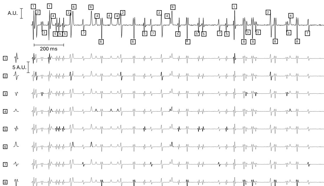
Fig. 3. Example of application of AWaRE to a simulated signal (including 8 waveforms, repeated 20 times in 10 s and including white Gaussian noise with SNR of 25 dB). The same parameters of AWaRE were used as in the previous Figures. Two seconds of the raw signal and the identified labeled waveforms are shown above, in the order of appearance (and of identification); single waveform trains are shown below for each of the waveforms (the 8 simulated waveforms are indicated on the left of each train).
