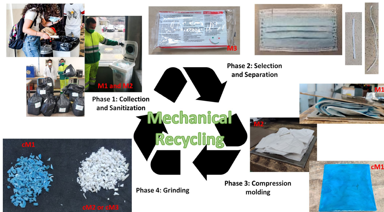
FIGURE 1 | Mechanical recycling phases of after use surgical masks (M1), FFP2 masks (M2), and new surgical masks (M3).
