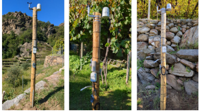
Figure 1: Examples of weather stations used to acquire the dataset; the leaf wetness sensor can be recognized in the lower part of the pole.
