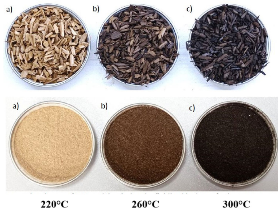
Fig. 1. Appearance of hemp hurd after the torrefaction process, before and after grinding. Torrefaction process was performed at (a) 220 °C, (b) 260 °C, and (c) 300 °C.
