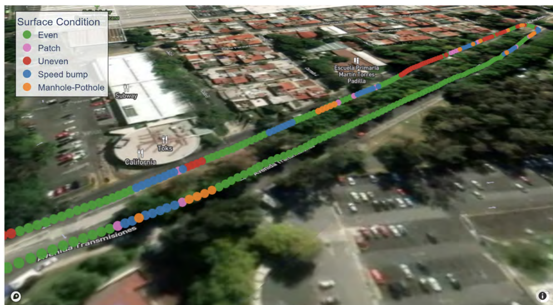
Figure 9. Spatial isolation of sequential speed bumps and manholes along a recently paved road surface.
