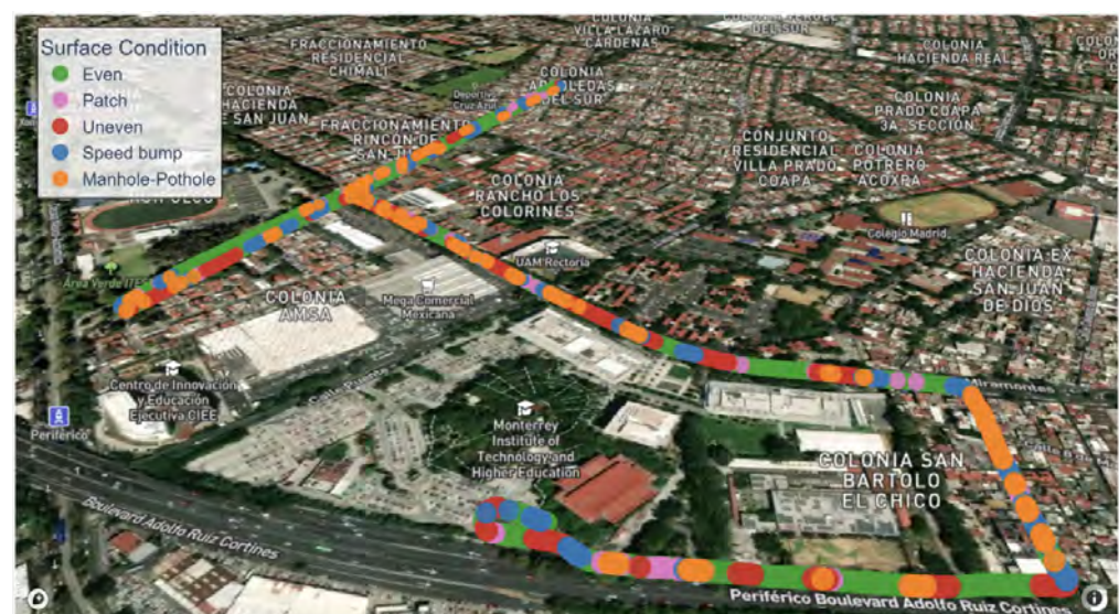
Figure 7. Geospatial map of the 3.75 km urban test route, plotting the continuous classification of road surface conditions generated by the real-time edge inference node.
