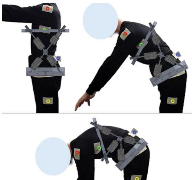
Figure 20b CAD visualization of exoskeleton worn by a 50 th ile Italian male volunteer.
