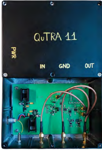
Fig. 7. Assembled QuTRA 1.1 PCB inside its box with the lid open. The amplifier interfaces via three SMA connectors (IN, OUT, GND) and a 4-pin LEMO connector for external battery supply.
