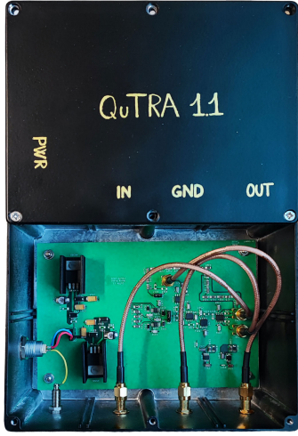
Fig. 7. Assembled QuTRA 1.1 PCB inside its box with the lid open. The amplifier interfaces via three SMA connectors (IN, OUT, and GND) and a four-pin LEMO connector for external battery supply.
