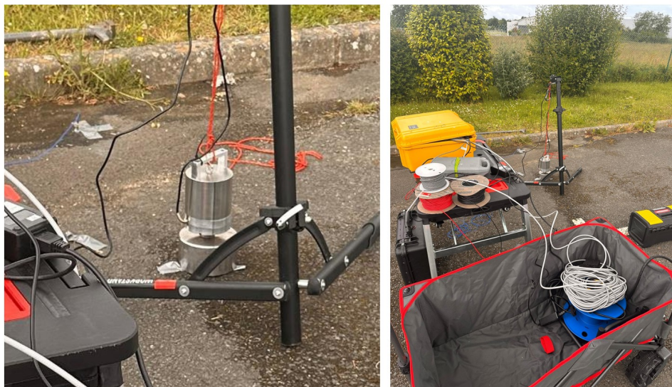
Fig. 4.6 Steel-to-Steel Concrete Test: One Meter from the Fiber Path.
