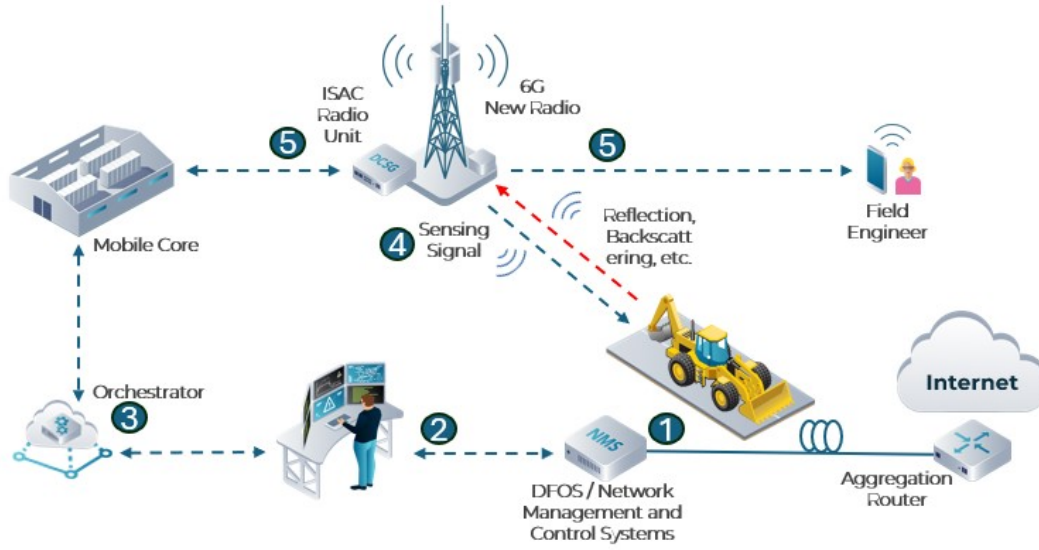
Fig. 2.4 Conceptual Diagram of ISAAC-DFOS Sensing System
