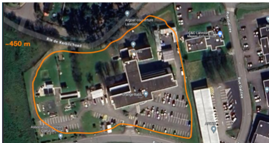
Fig. 4.1 450 meters Underground Deployed Dark Fiber Link
