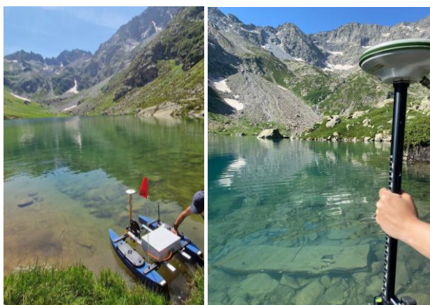
Figure 3. BlueBoat USV, BlueRobotics, equipped with STX-Echos Echosounder (left); point acquisition on shallow water through GNSS receivers for validation (right).
