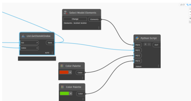
Figure 16. Dynamo script showing the connection of the Python script and its inputs to change the colours of the selected element in the model.
