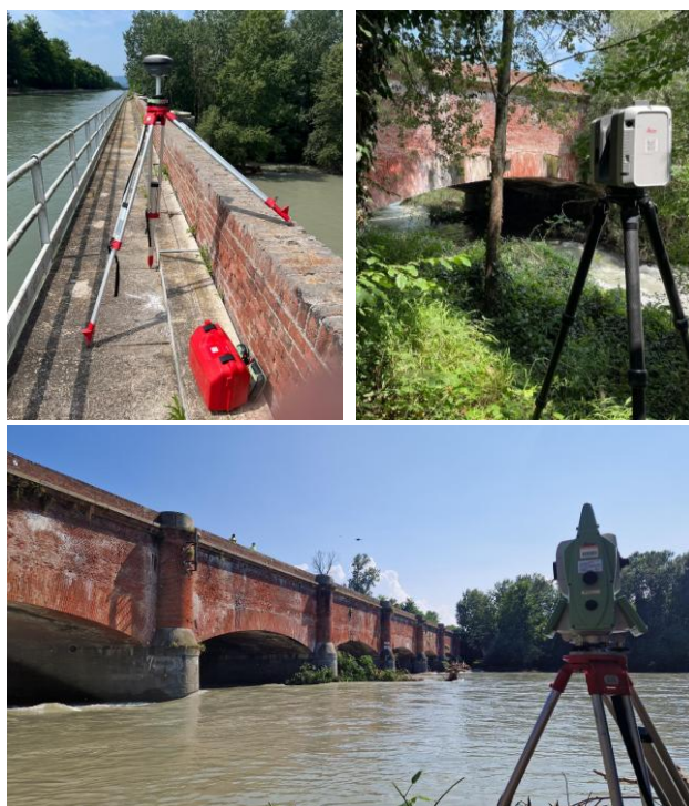
Figure 4. Data acquisition with Leica GS18, RTC360 and Leica MS50 (March 2025).
