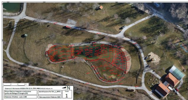
Figure 7. Orthophoto of the study area with superimposed spot heights acquired through traditional topographic survey
