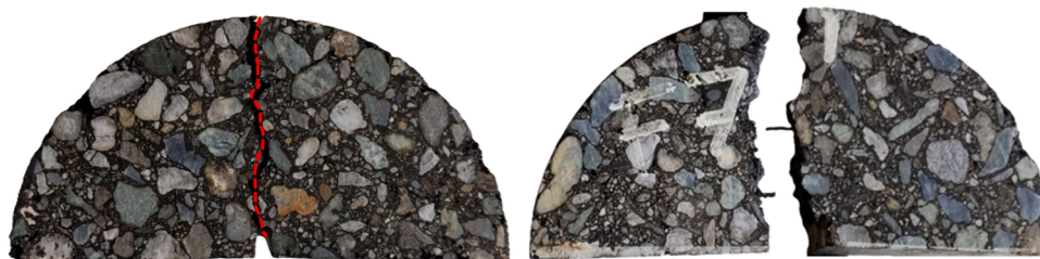
Fig. 7. Example of crack growth (left) and WTSF filaments observed on fractured surfaces (right) after SCB tests.
