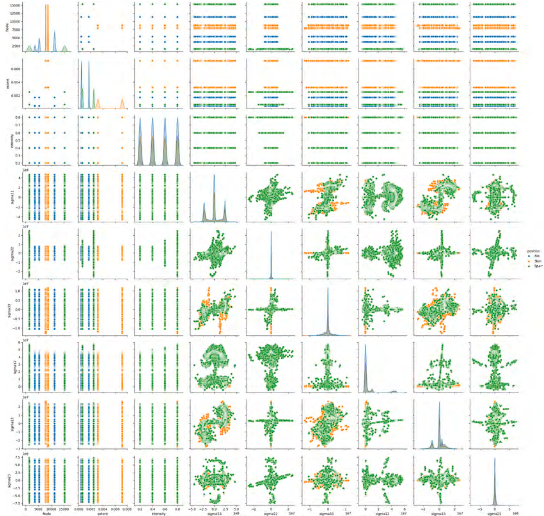
Fig. 8. Scatter plots of damage variables versus stress tensor, color-coded by categorical position.
