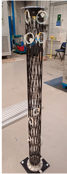
(a) Picture of the LRBOOM with fiber-optic strain sensors installed. The top metallic flange present in this picture is not modeled because it is not part of the composite structure investigated in the study.
