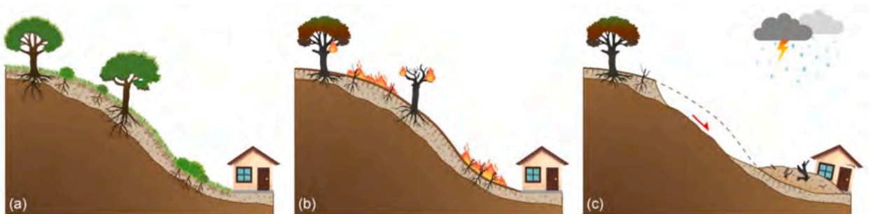
Fig. 8. Evolution of a slope affected first by wildfire and subsequently by rainfall, leading to instability. (a) Pre-fire condition: slope covered by soil and vegetation. (b) Wildfire event with varying burn severity, causing alterations in soil and vegetation. (c) Post-fire rainfall triggering a shallow landslide, with consequent damage to the built environment.
