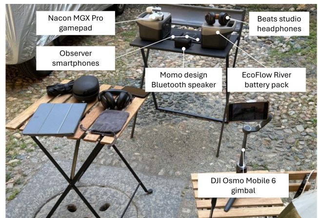
Fig. 6. Configuration for the crowded Bluetooth experiment.
