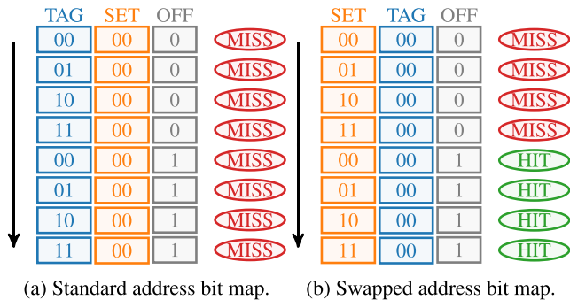
FIGURE 10. MatMult : sequence of addresses of B accessed during the first 8 iterations, where B \in \mathbb{R}^{4 \times 8} has a 4-set direct-mapped cache.
