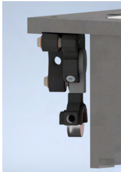
Fig. 6.6 Provisional kinematic mount for the bow-tie mirrors alignment.
