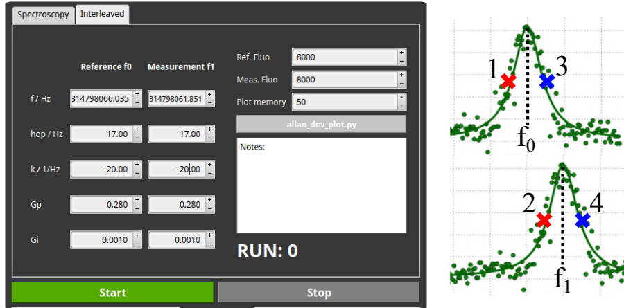
Fig. 3.24 Clock interleaved operation settings within the control graphical interface. From this panel, the expected center frequencies of the resonances f_0 (reference) and f_1 (measurement), the detuning at which the interrogation happens (hop) and the loop gains can be set. The right side of the figure shows conceptually the procedure of the interleaved operation. Red-detuned side interrogation of the reference (1) and measurement (2) excitation profiles, blue-detuned side interrogation of the reference (3) and measurement (4) excitation profiles.
