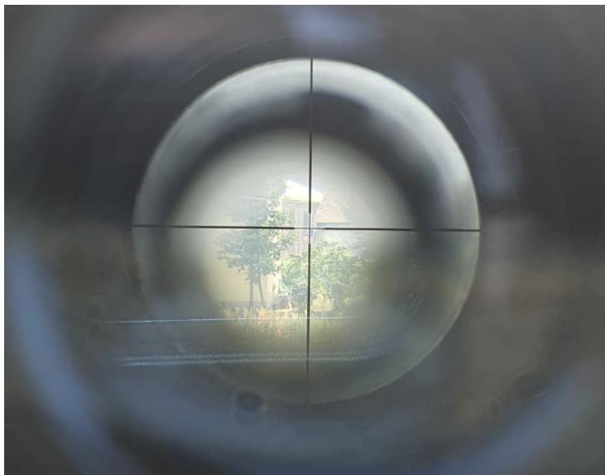
Figure 89: View through the telescope mounted on the transmitter towards the receiver.
