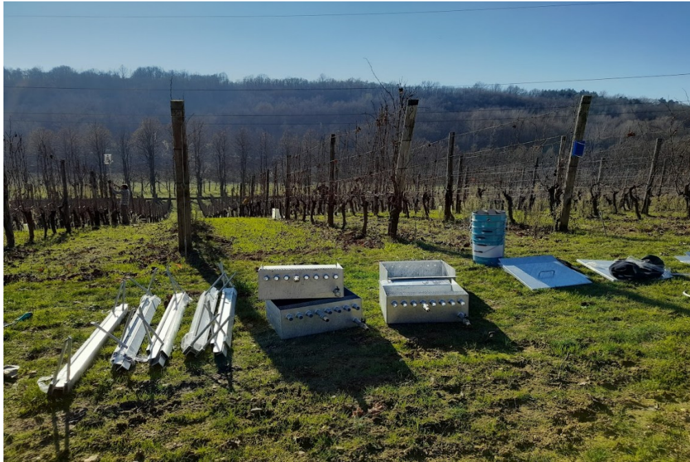
Figure 17: Components for the realization of the runoff and erosion measurement system in the vineyard (at Biné vineyard, Novi Ligure): bars for the delimitation of micro-plots and Gerlach-type tanks with dividers and lids (made of galvanized iron), and tanks with holes for the collection of runoff.
