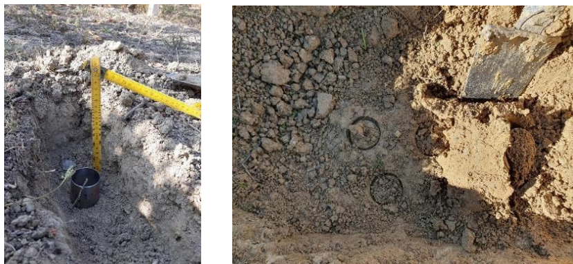
Figure 49: Sampling in the vineyard for measuring soil bulk density and soil water content.
