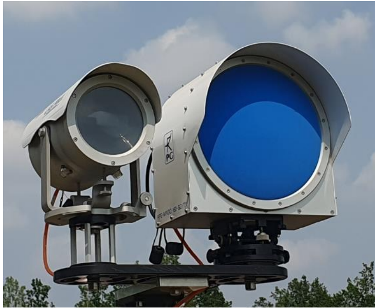
Figure 86: The optical and microwave scintillometers (transmitting units)
