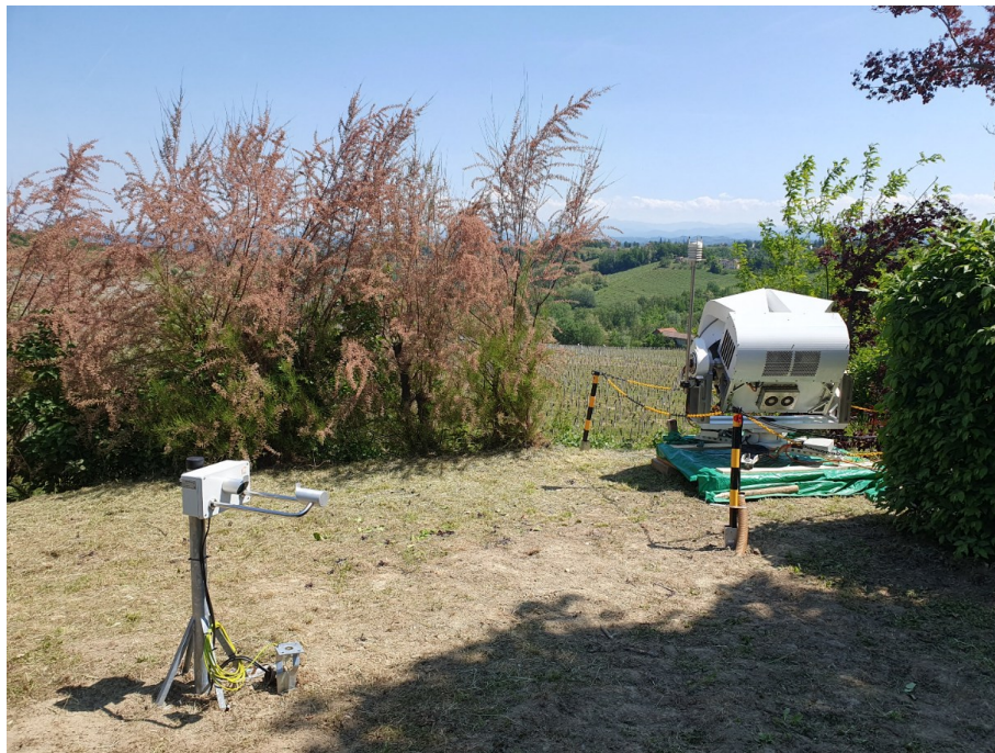
Figure 75: The disdrometer on the left and the radar on the right, installed in position.
