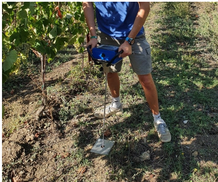
Figure 57: Execution of a penetrometer test to determine soil penetration resistance.
