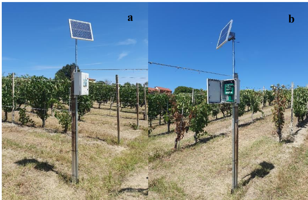
Figure 100: Instrument and solar panel installed on the pole (a) and with the protective box open (b).
