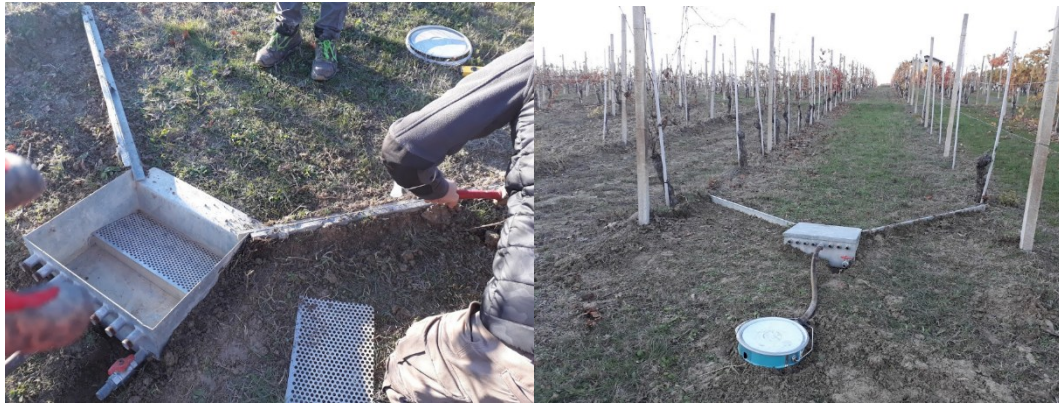
Figure 18: Installation of runoff measurement systems (tanks and delimitation bars with second tank) at Tenuta Cannona, Carpeneto.
