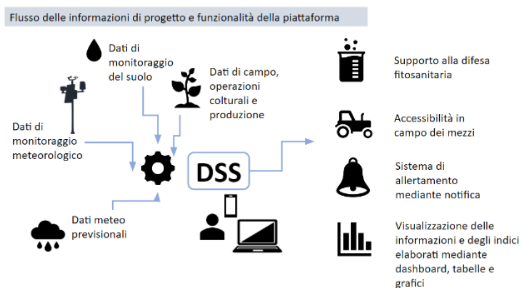
Figure 45: Schematic representation of the DSS powered by the monitoring system, which provides useful guidance to technicians and viticulturists for phytosanitary protection and field accessibility.
