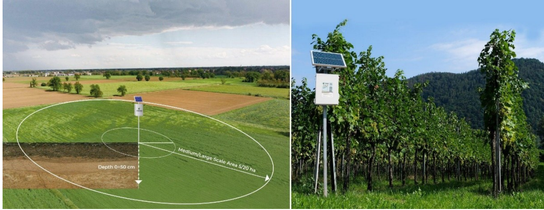
Figure 108: On the left scheme of the CRNS footprint, on the right the Finapp probe installed in a vineyard.
