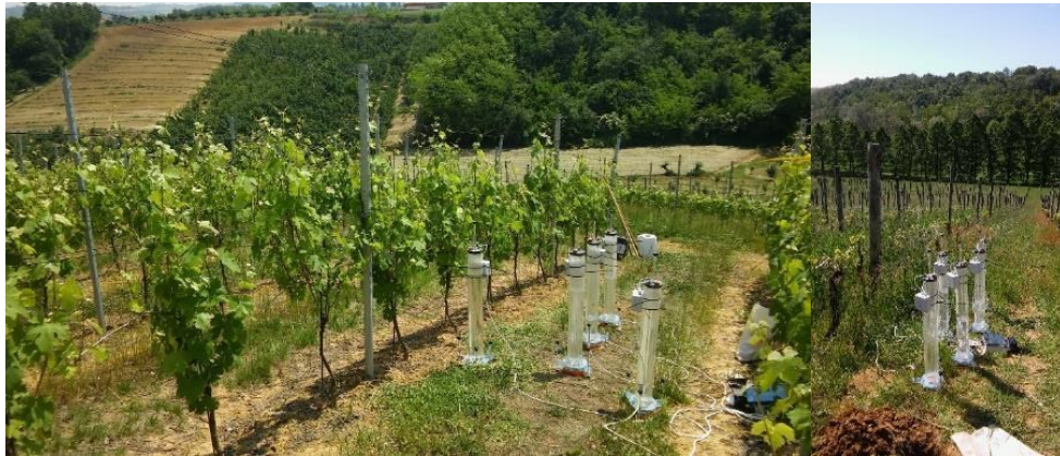
Figure 61: Execution of infiltration tests in vineyards to determine saturated hydraulic conductivity.
