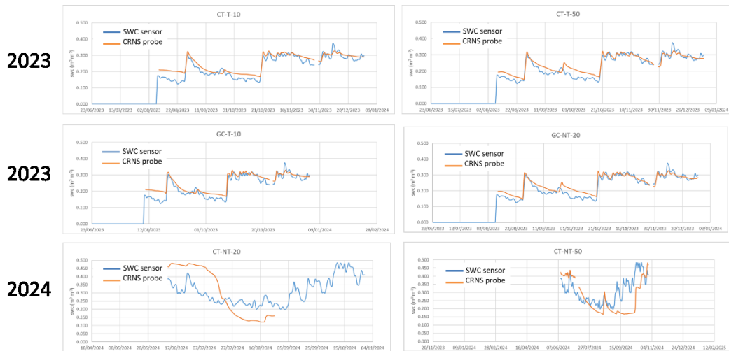
Figure 104: Comparison of the daily average Soil Water Content (SWC) obtained from point capacitive sensors and CRNS (best performing sensors).
