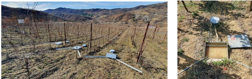
Figure 23: On the left, the Gerlach microplots installed in the rows of the Rocchetta Ligure vineyard. On the right, the Gerlach tank after collecting runoff water and sediments.
