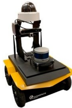
Fig. 5.4 The Jackal platform, equipped with a ZED2 stereo camera, used in this work.
