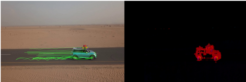
Fig. 2.1 An example of a Sparse OF field (on the left) and a Dense OF field (on the right).
