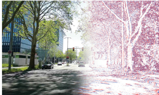
Fig. 1.1 Comparison between frame-based (on the left) and event-based cameras (on the right): the event-based output highlights motion while reducing redundancy. Picture taken from the website of the Robotics and Perception Group, University of Zurich, Switzerland.
