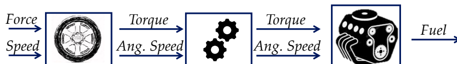
Fig. 3.6 Information flow in a backward kinematic approach.
