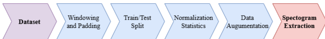
Figure 5: Preprocessing Data Pipeline.
