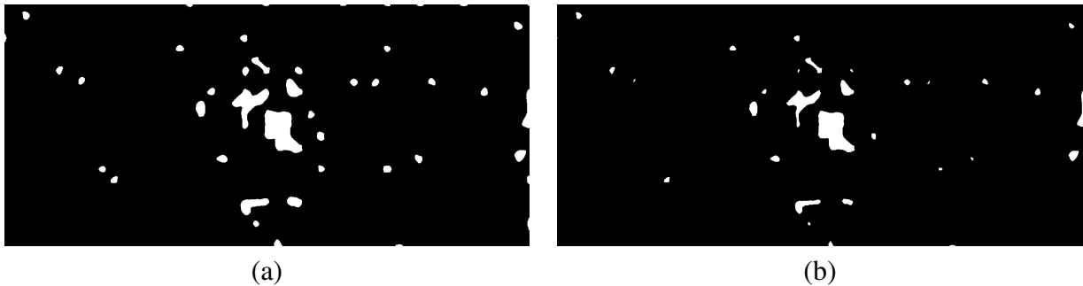
Figure 3: (a) Damage Mask after completion of phase 2; (b) Damage Mask after the application of Erode kernels.
