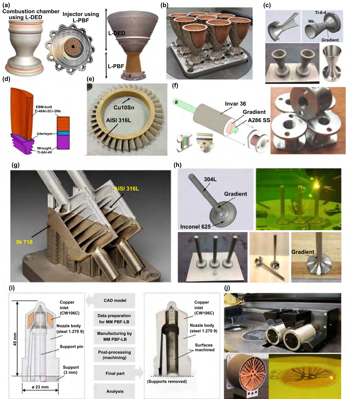
Figure 12. Examples of multi-material with potential applications in the aerospace and automotive sectors. (a) Examples of component configurations using Copper-Superalloy bimetallic AM. From [298] . Reprinted with permission from AAAS. (b) Nickel-Copper combustion chambers (Fraunhofer IGCV). Reproduced with permission from [301] . © Fraunhofer IGCV, Prof. Christian Seidel. (c) A one-piece rocket made of low-density Ti6Al4V and high-melting temperature refractory metal (Nb). Reproduced from [302] , with permission from Springer Nature. (d) Ti48Al2Cr2Nb and Ti6Al4V bimetal component. Reprinted from [303] , Copyright (2021), with permission from Elsevier. (e) L-PBF-manufactured AISI 316L-Cu10Sn for aircraft turbine disk. Reproduced from [284] . © 2020 The Author(s). Published by IOP Publishing Ltd on behalf of the IMMT. CC BY 3.0 . (f) A286 SS to Invar36 gradient alloys for carbon fiber composite inserts. Reproduced with permission from [304] . CC BY-NC-ND 4.0 . (g) Aerospace heat exchanger AM using stainless steel SS316 and Inconel 718. Reprinted from [219] , Copyright (2021), with permission from Elsevier. (h) The fabrication of SS304L to IN625 automotive valve stems. Reproduced from [302] , with permission from Springer Nature. (i) An injection nozzle for large bore engines, investigated in cooperation with MAN Energy Solutions SE (Prof. Christian Seidel (Munich University) Fraunhofer IGCV). Reproduced with permission from [301] . © Fraunhofer IGCV, Prof. Christian Seidel. (j) Multi-material heat sink additively manufactured in a copper alloy (inner core) and stainless steel (outer shell) investigated in Aerosint, worked with the Fraunhofer [305] . Reproduced with permission from [306] . © Schaeffler Aerosint SA.
