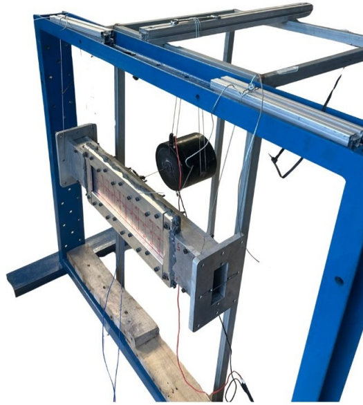
Fig. 3 Modal analysis test rig.
