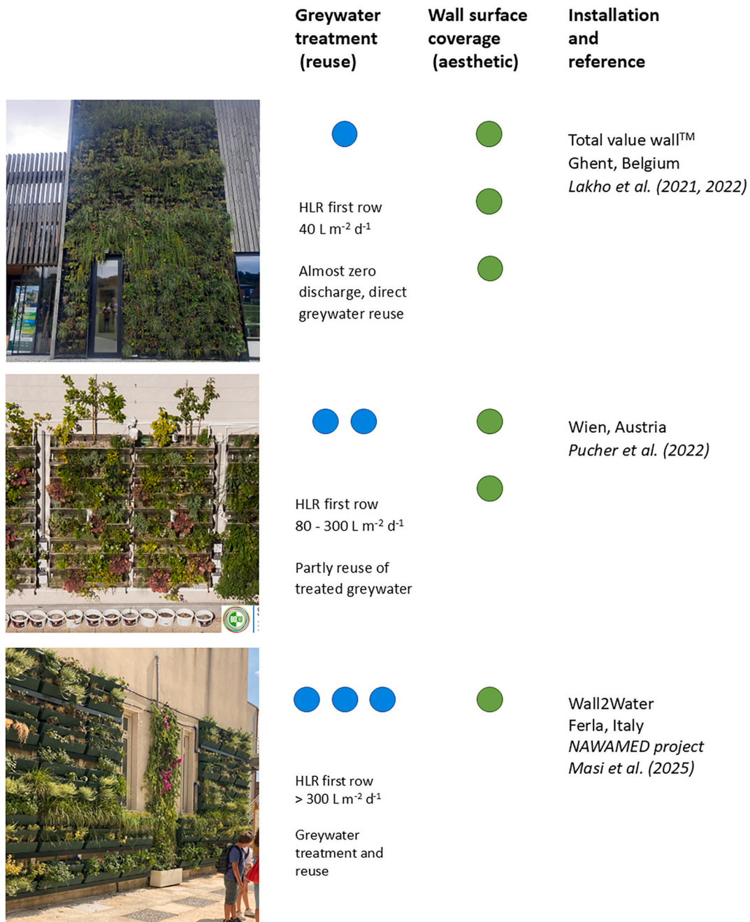
Fig. 3. Overview of alternative design approaches for balancing different ecosystem services of green walls proposed in literature. Dots show the importance of a specific service for each configuration.
