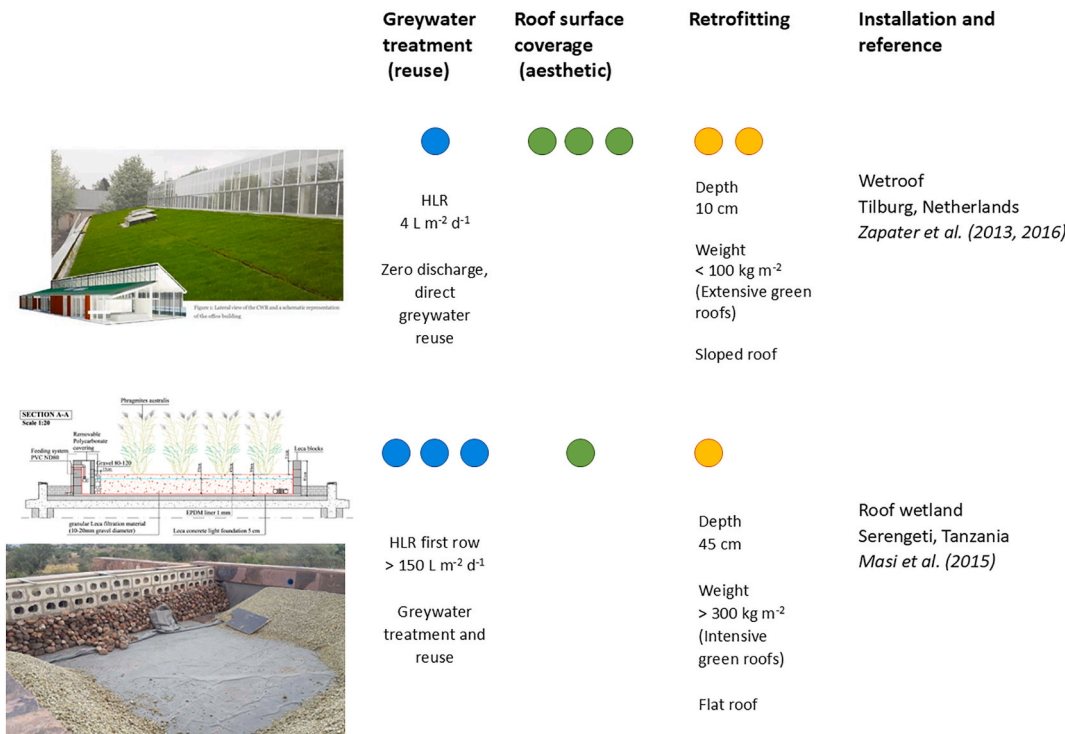
Fig. 4. Overview of alternative design approaches for balancing different ecosystem services of green roof proposed in literature. Dots show the importance of a specific characteristic for each configuration.
