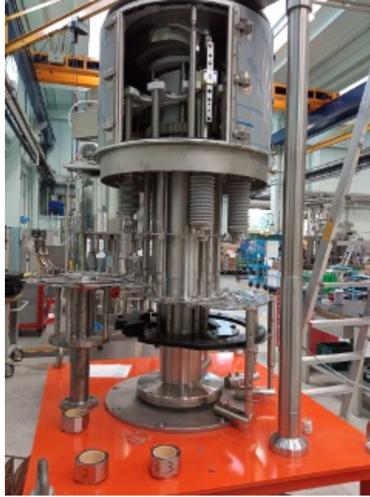
Fig. 5.1 Capping Machine sensorized with ISM330DHCX IMU
