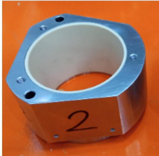
Fig. 5.2 Slightly worn bush
