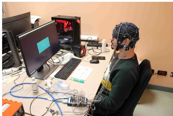
Fig. 4. Photography of the experimental setup and subject position during the experiment. On the screen it is shown the command for the rest state, a blue rectangle in the middle of the screen.
