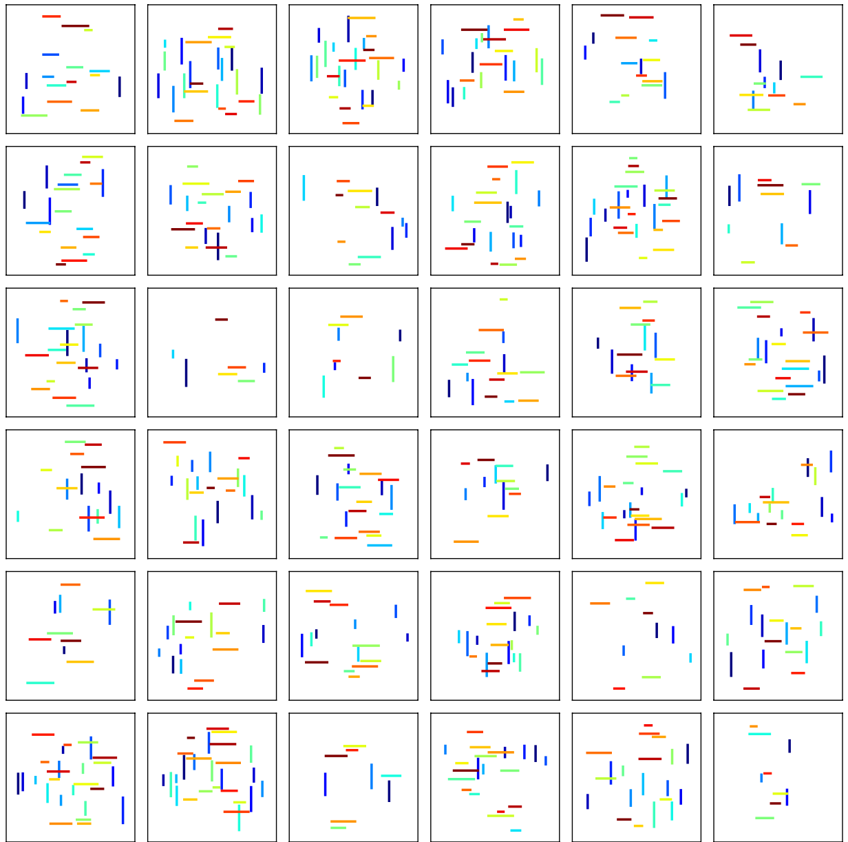
Fig. 3 Examples of randomly generated initial fracture patterns with orthogonal orientations used in fracturing simulations. Colors in the plots represent distinct fractures. The size of the simulated domain is H_x = H_z = 0.25 m (omitted for brevity).
