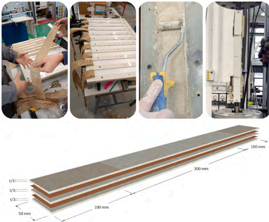
Fig. 5. Production, testing and schematic representation of the Natural TRMs.
