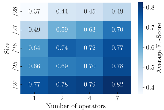
Fig. 6. Average F1-Score when embeddings are generated through the FL collaborative between an increasing number of operators using dataset (b).
