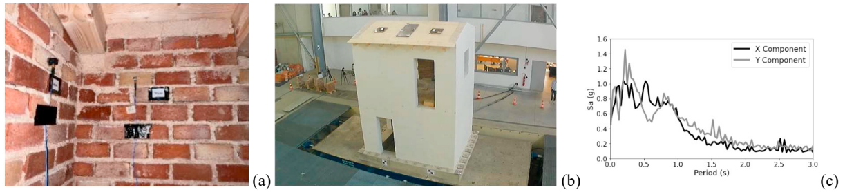
Fig. 5. (a) View of the sensors installed in the inner sides of the walls; (b) Overall view of the specimen in the shake table; (c) Response spectra of the reference input earthquakes.
