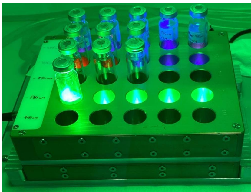
Picture 1. The photoreactor used for the photoreactions is equipped with five LED lines, with different wavelength emissions. Reprinted with permission from ref 58. Licensed under CC-BY 4.0. Copyright © 2025 The Authors.
