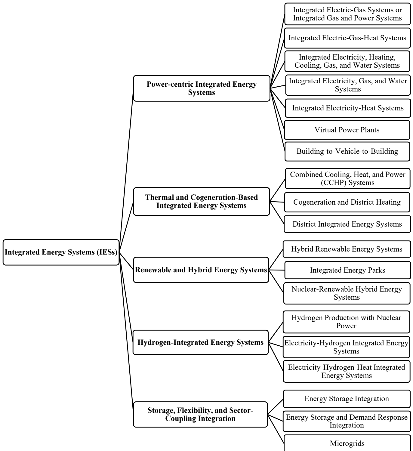
Figure 1. The most common types of integrated energy systems (IESs) and their categories.
