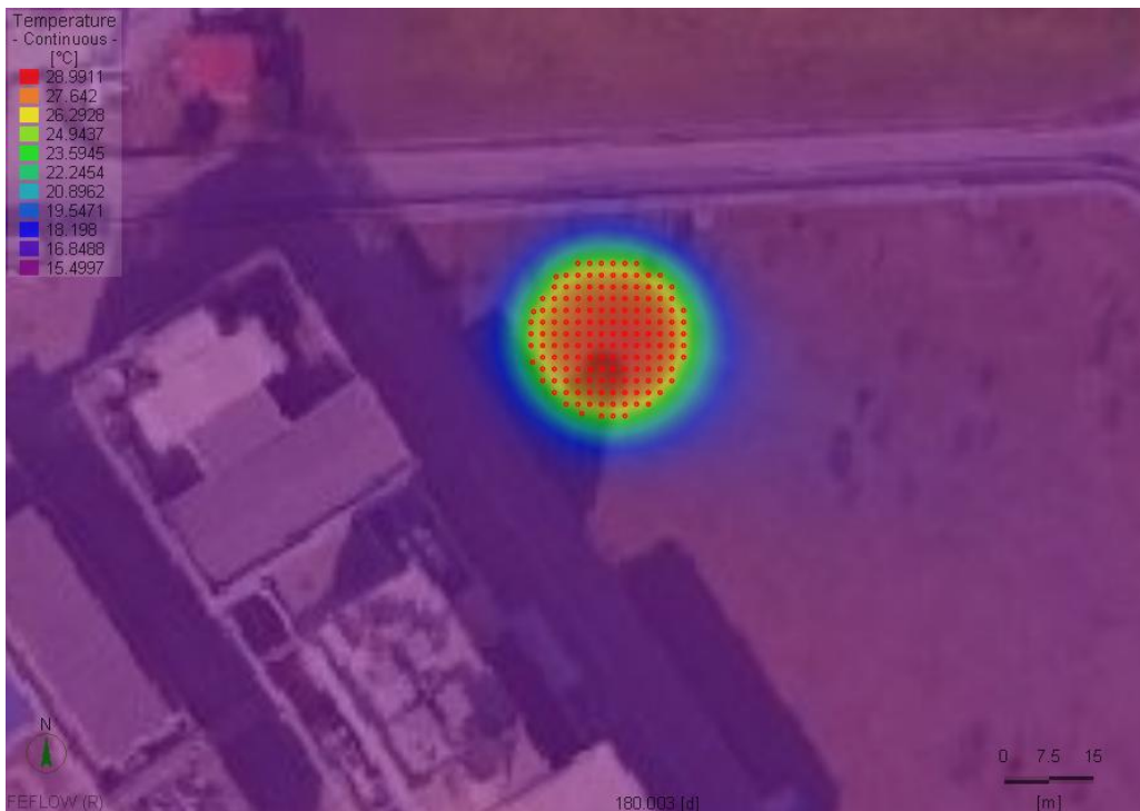
Figure 159. Thermal interference of the BTES system in horizontal section at the end of the fifth charging period.
