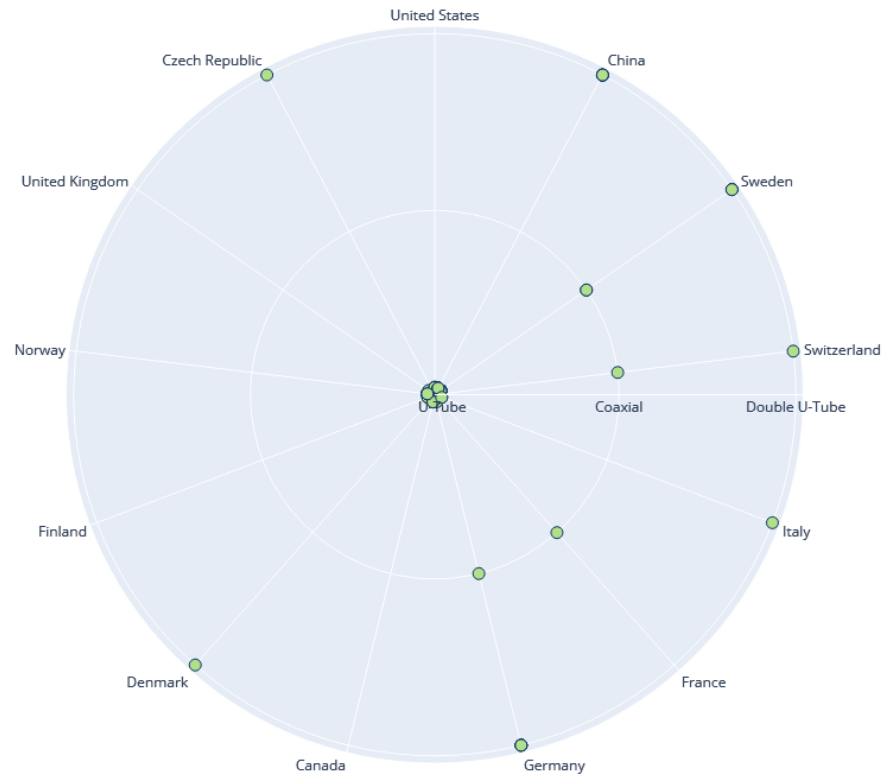
Figure 144. Polar Plot of type of tubes utilised in BTES in the different countries.
