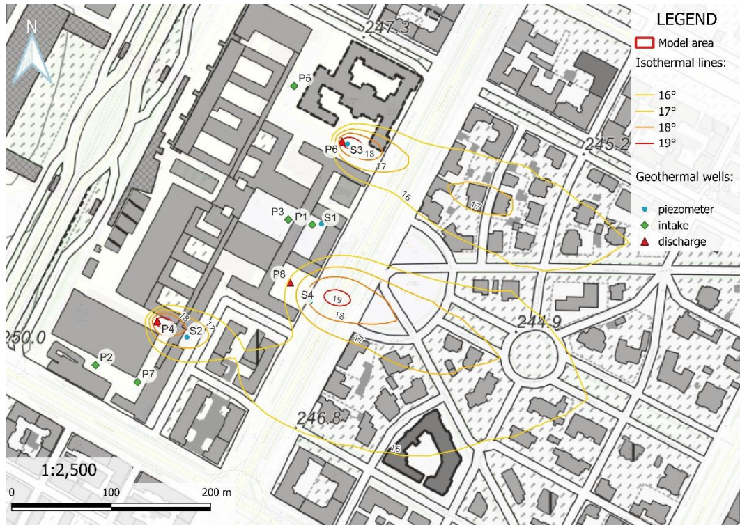
Figure 68. Thermal plume simulation of the main campus at the end of August 2024.
