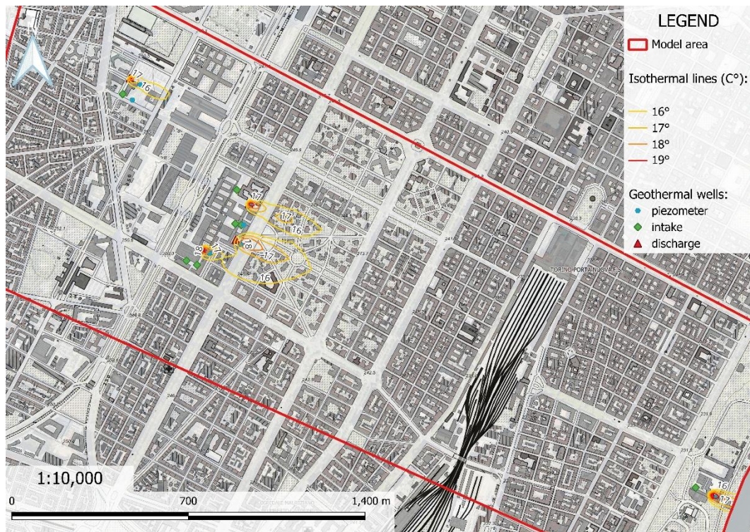
Figure 67. Thermal plume map of the study area representing the geothermal plants simulation at the end of August 2024.
