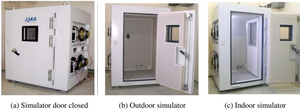
Fig. 1.10 JAXA indoor and outdoor sonic boom simulators [3]
