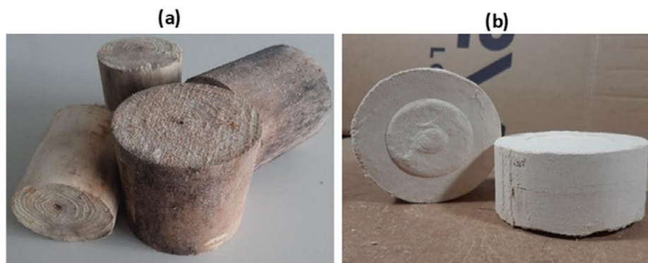
FIGURE 12 | Raw poplar wood P_I (a) and briquettes P_{IV} (b).
