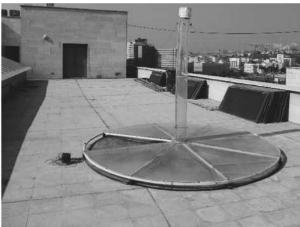
Fig. 10. Experimental set-up of the model-scale solar chimney [78].
