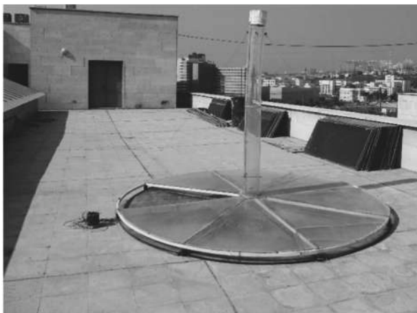
Fig. 10. Experimental set-up of the model-scale solar chimney [78].
