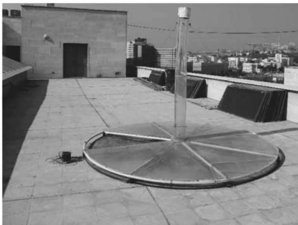
Fig. 10. Experimental set-up of the model-scale solar chimney [78].
