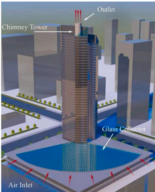
Fig. 25. The visualization of SCPP integration with a high-rise building [132].
