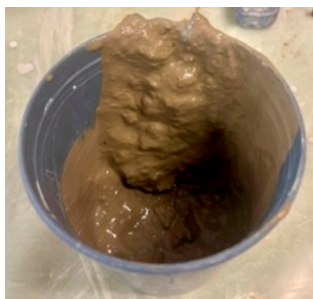
Figure 6. Result of the gel time test for WBS ID 1.
