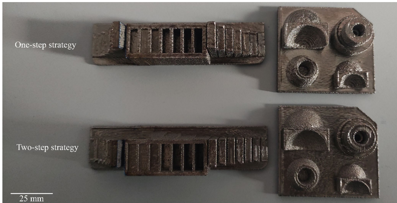
Fig. 4 Samples produced using the one-step and the two-step strategy
