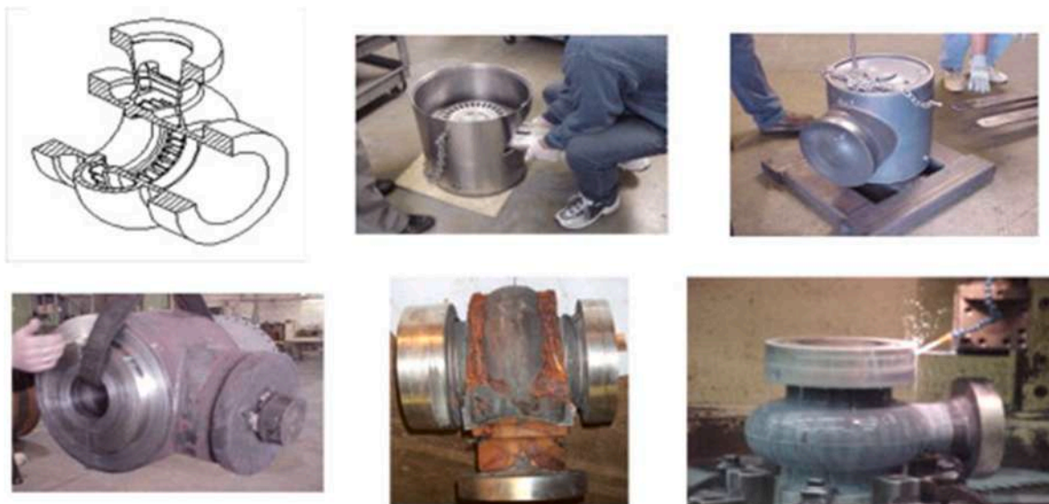
Fig. 14. Titanium engine housing fabricated via NNS-HIP [14].
