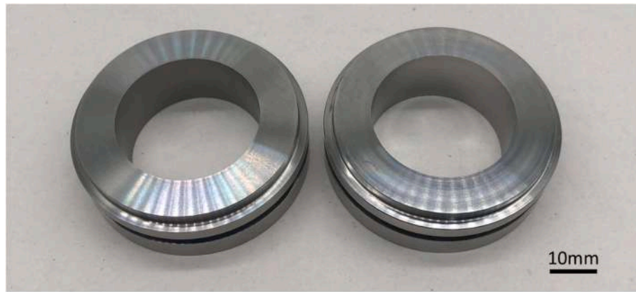
Fig. 16. Ni-MMCs mechanical seals after machining produced by NNS-HIPping [128].
