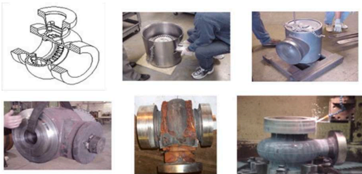
Fig. 14. Titanium engine housing fabricated via NNS-HIP [14].
